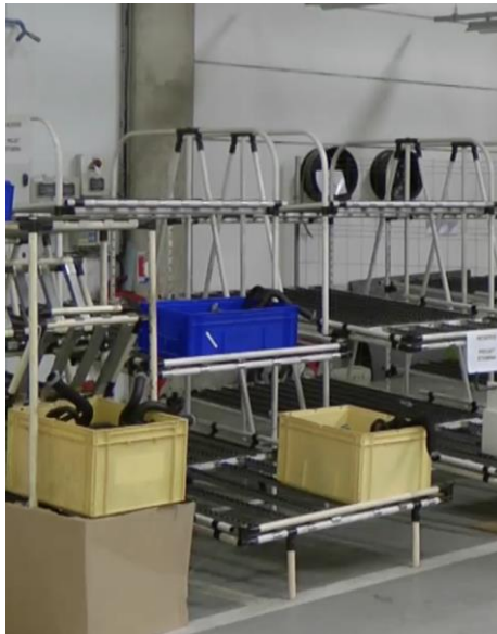
Figure 4 shows how tubes are stored in the boxes and how boxes are placed on the racks
