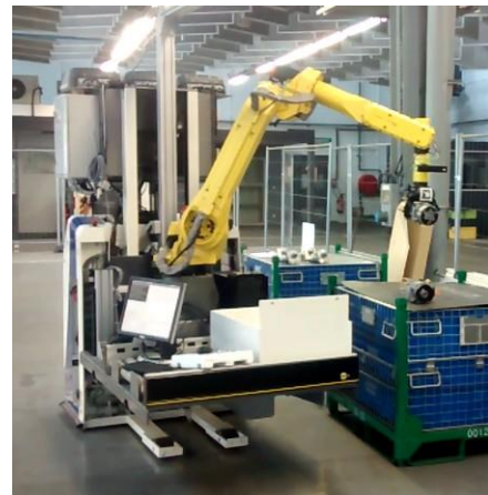
Figure 1: A robot operating in a factory environment using the SkiROS system. The robot is executing a six-step plan to place two parts in the white kitting box it is carrying.
