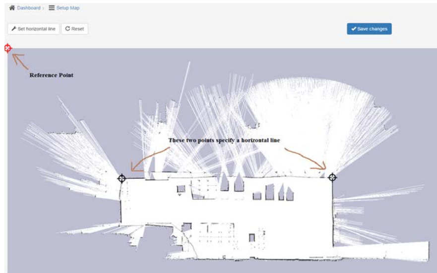
Figure 14 – User interface: reference point and horizontal line on a SLAM-based image.
