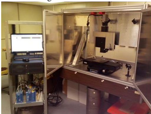
Figure 3: Workstation for the TiSa laser systems.
