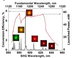
This was achieved by using a method called second harmonic generation (or frequency doubling), where effectively an infrared wavelength is converted using a crystal (in this case periodically poled KTP) into visible wavelengths.
