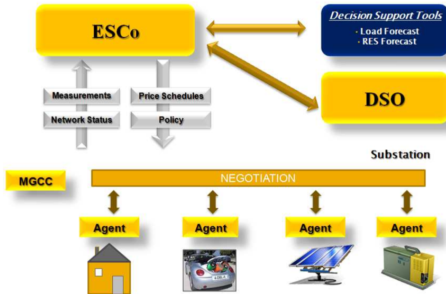
Figure 6: Schema of the MAGIC technology
