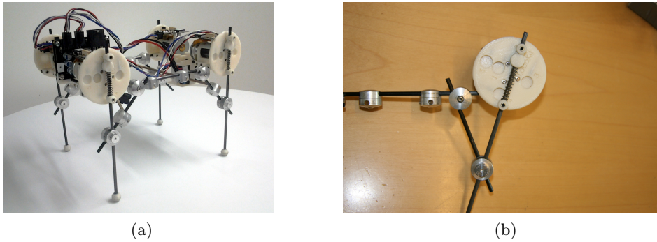
Figure 1.1: (a) latest version of the SpringyBot and (b) crank-slider mechanism implementation of the SpringyBot
