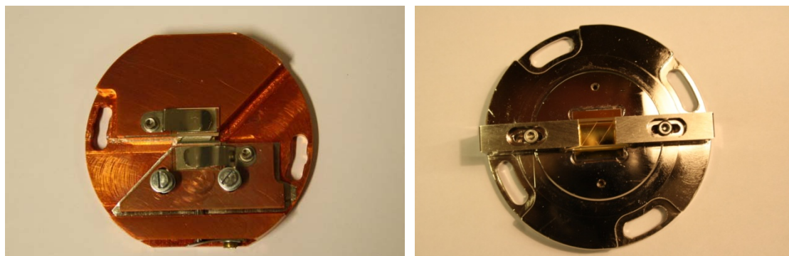
Fig. 14. Different laser crystal clamping methods. Left: side clamping. Right: top–bottom clamping. The conductive cooling from the top in the configuration on the right is supplied via an AR-coated sapphire prism which is bonded on an optical contact to the gain crystal. The cooling from the bottom is provided by a Au-pated diamond plate soldered to the copper heatsink. The model on the left shows a newer, 1.5×1.5 mm cross-section crystal, whereas the model on the right shows the original 5×1.5 mm type. The diameter of the outer disk is 70.6 mm.
