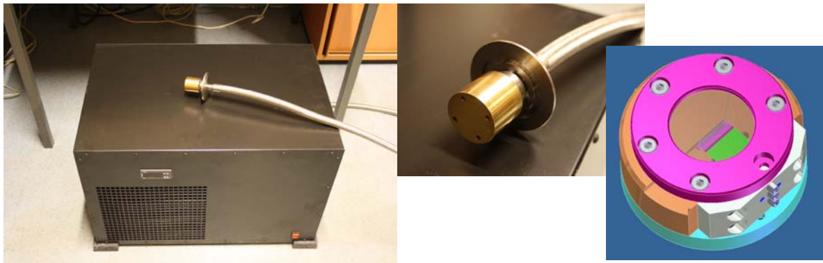
Fig 20. 150 W 130 K JT cooler developed at TU WIEN. Insets show the photograph of the cold head that is flanged to a chamber using an ISO KF 50 flange. The inset on the right shows the design of a specially adapted crystal holder that should enable adjustable crystal clamping on four sides and minimize the exposure of the heatsink to ASE radiation.
