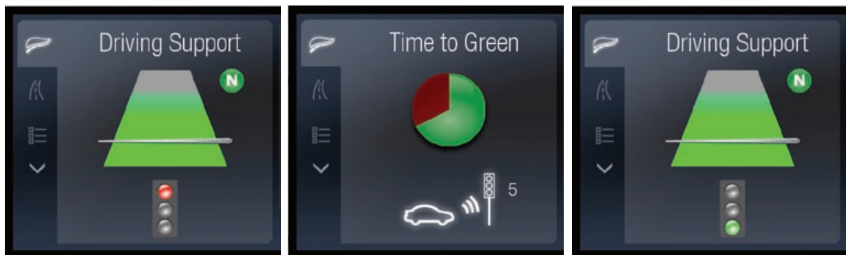
HMI examples for the ecoDrivingSupport function
