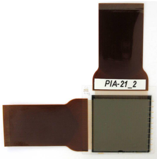
Figure 15: Display module with bonded FPCs and crossed polarizing filters. Image copyright owned by Asulab.
