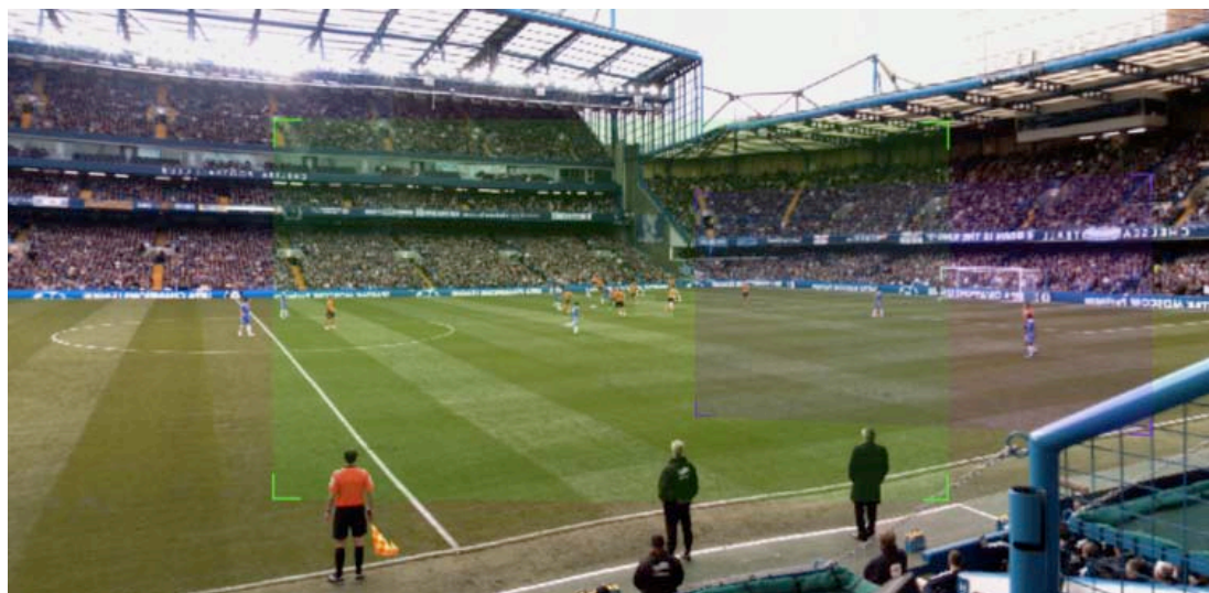
Figure 4: In test content from a soccer match, Technicolor's FRN renderer visualizes shot candidates as computed by the Production Scripting Engine as coloured overlay rectangles.
