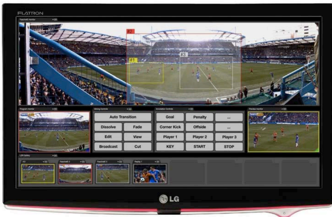
Figure 8: Production Control Workspace of the Editor User Interface, including panoramic overview, virtual camera control and high level annotation controls.
