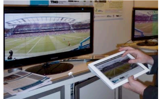
Figure 6: prototype of a delivery network based on spatially segmented content, that allows for second-screen pan/tilt/zoom interaction.
