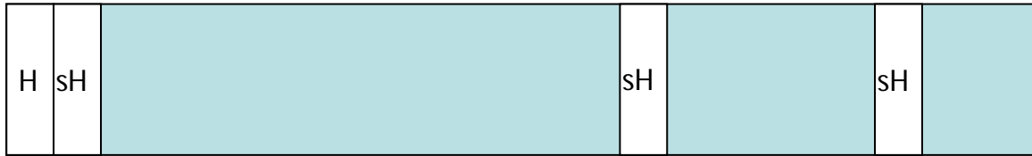
Figure 4-2 Serialized transport of LSR subparts. A global header H describes all necessary information for parsing the packet in a hierarchical way, sub headers sH describe each subpart identification data and payload size. Blue parts are LSR subparts in raw format
