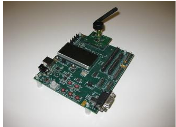
Figure 7: a) Reprogramming the TI CC2530 in the lamp b) TI SmartRF Evaluation Board
