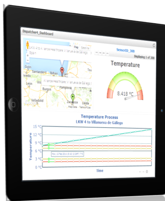
Figure 27: Dispatcher Dashboard showing truck position with temperature values
