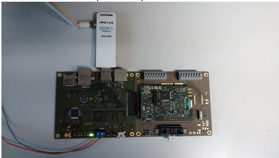
Figure 21: Urban Security use case – ARAGO WisCore wireless platform picture
