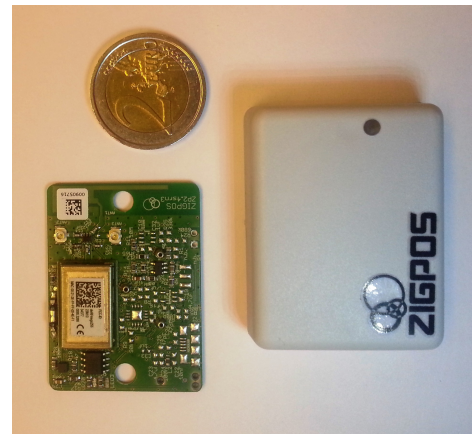
Figure 47: Wireless sensor node used in the Smart Hospital trial: (a) hardware architecture and (b) photo of the node.
