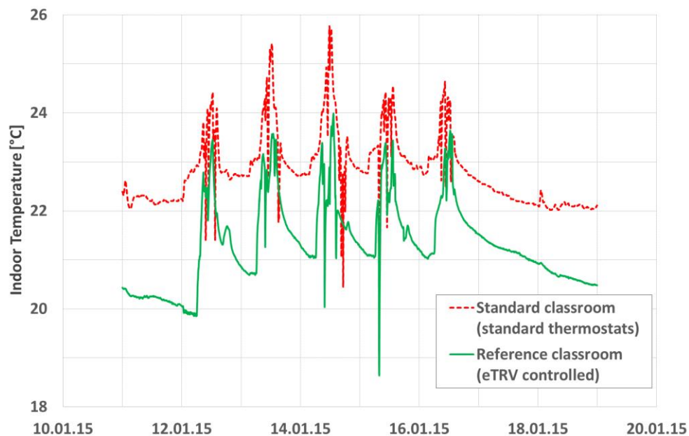
Figure 9. Temperature profiles of two classrooms in comparison. Green line: room with ICT controlled heating on room level. During occupancy periods indoor room temperatures are kept at a defined level. During non-occupancy temperatures are regulated down; Red line: room with manual control based on standard thermostats (normally thermostats are turned by pupils on maximum). Temperature levels do sometimes reach high uncomfortable levels. As a consequence windows are opened.
