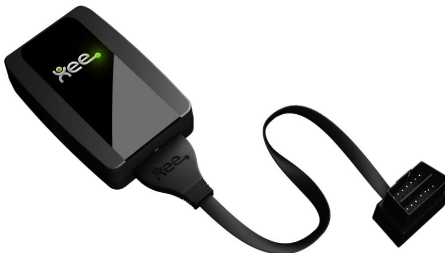
Figure 4-1 BlueDash "DQuid Xee" on-board unit for Reggio Emilia pilot site
