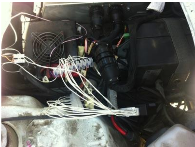
Figure 101: Data Acquisition System installation (2)
