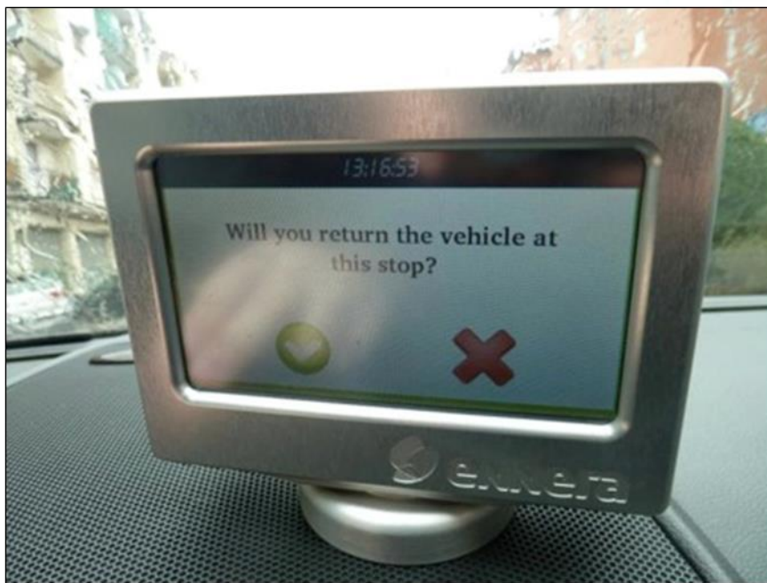
Figure 48: The OBU ask to the driver for the confirmation of the return.
