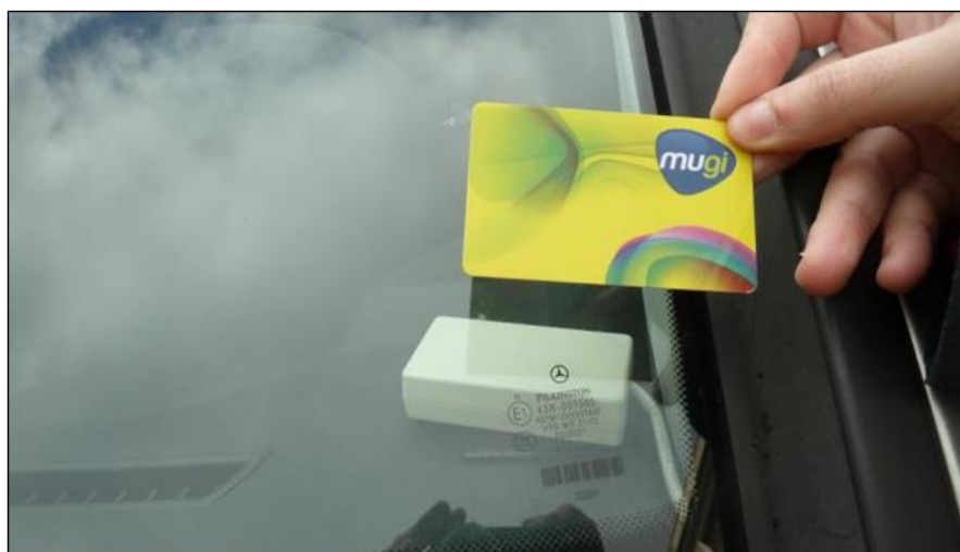
Figure 51: The driver closes the vehicle using the user card in the RFID reader.
