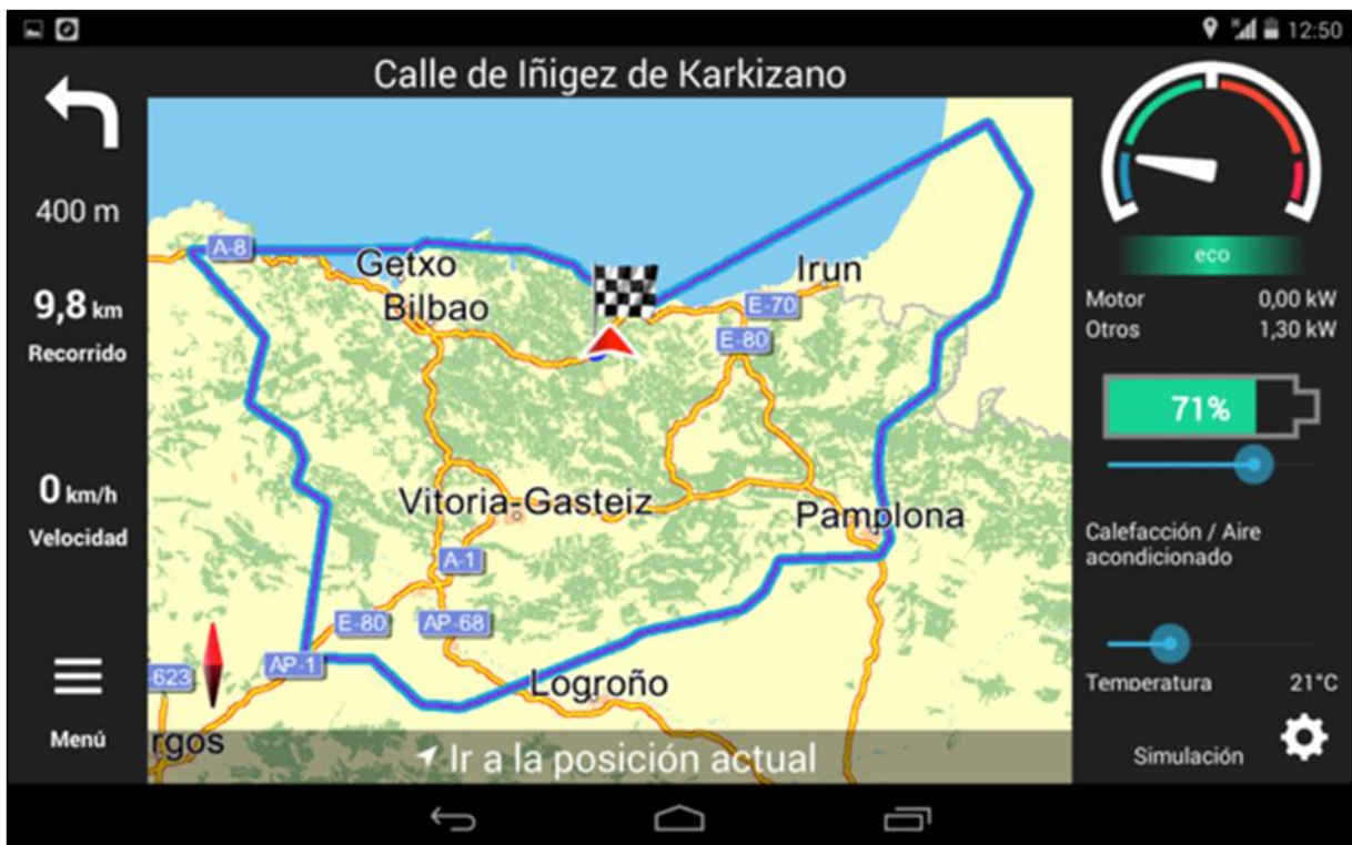
Figure 42: The allowed range according with the current battery charge in the EV-Navigation system.
