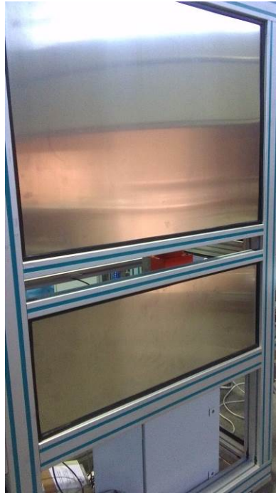
Fig. 5: Shades of the registration Module to prevent errors caused by illumination and daylight
