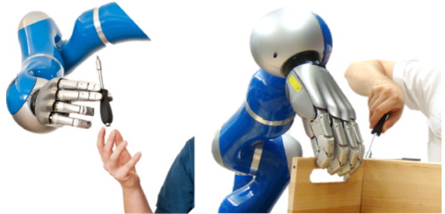
Fig. 1. Illustration of two collaborative tasks where a semi-autonomous robot helps a worker assembling a box. The robot must predict what is the action to execute, to hand over the screw driver or to hold the box. Its movement must also be coordinated relative to the location at which the human worker executes the task.
