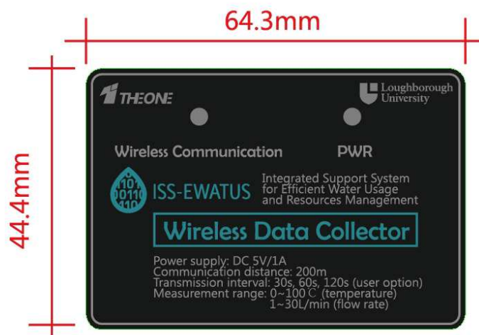
Figure 8. Panel layout of the wireless data collector
