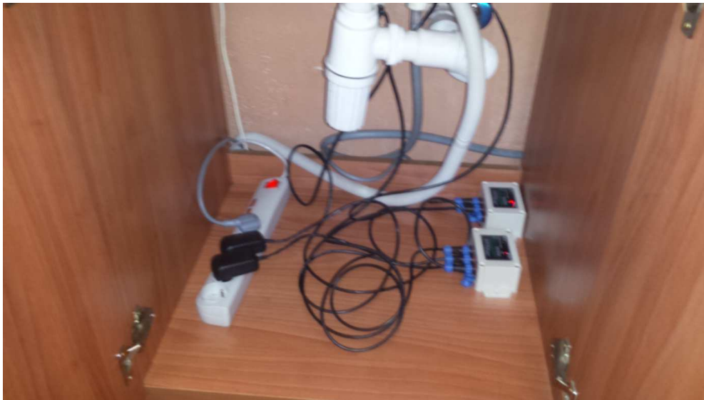
Figure 14. Flow sensors are connected to data collector nodes (one collects data from the tap and second from the dishwasher), nodes are mains powered
