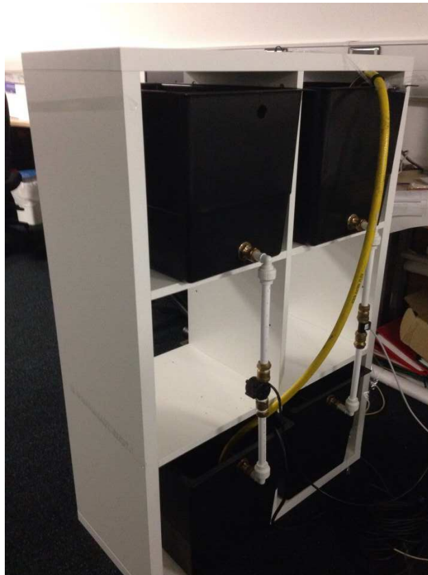
Figure 2. Test rig for water consumption monitoring at Loughborough University
