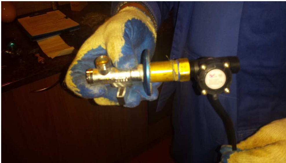
Figure 12. Flow sensor is mounted on the hydraulic adapter
