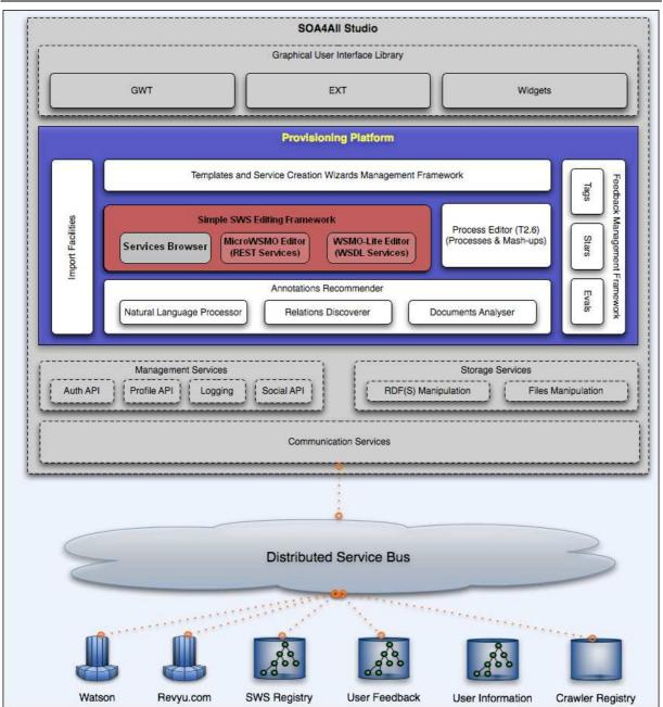
Figure 2: Service Provisioning Platform architecture overview
