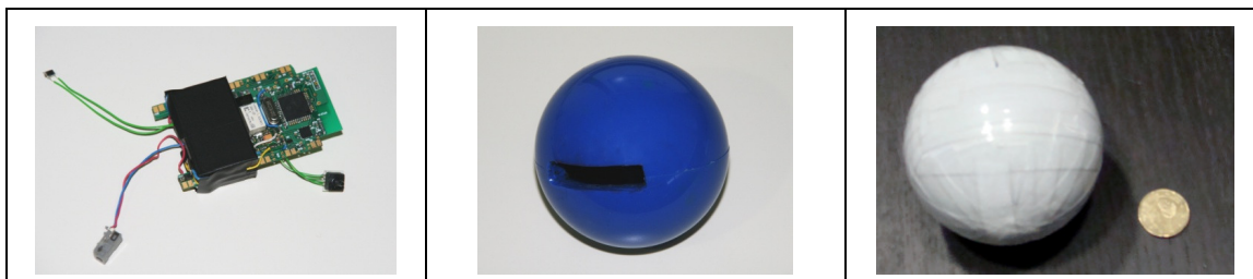
Figure 4: The Squeezy Ball interaction device: left: sensors, center: shell, right: final 1 st prototype.
