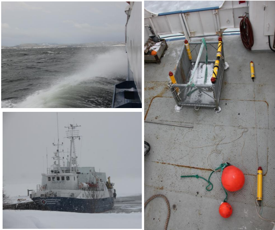
Figure 7 Modem range test scenario and equipment 3 including all 6 UAN modems
