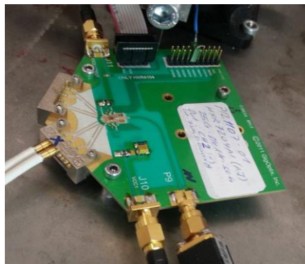
Figure 30. Evaluation board for the 25 Gbit/s driver with electrical input and electrical output.
