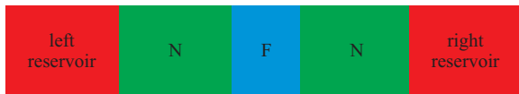
FIG. 1: Schematic picture of a ferromagnet (F) in contact with a thermal bath (reservoirs) via metallic normal metal leads (N).
