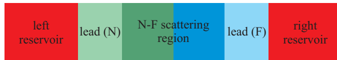
FIG. 3: Schematic of how transport between a normal metal and a ferromagnet is computed by scattering theory. The scattering region, which may contain the normal metal-ferromagnet interface and diffusive parts of the normal metal as well as ferromagnet, is attached to real or fictitious leads that are in contact with a left and right reservoir. In the reservoirs, the distributions of charges and spins are assumed to be known via the charge potential and spin accumulation bias.
