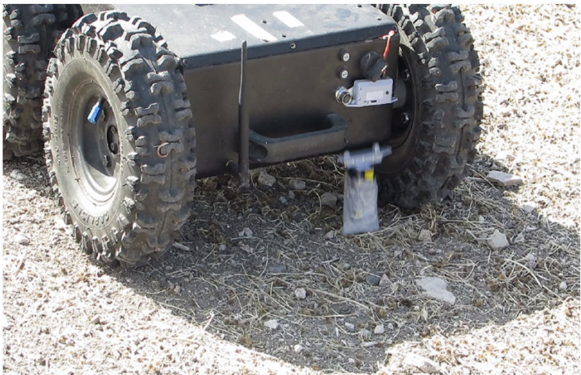
Figure 4: UGV dropping a sensor.
