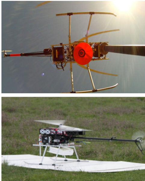
Figure 34: Helicopters as CO deployment and retrieval tools
