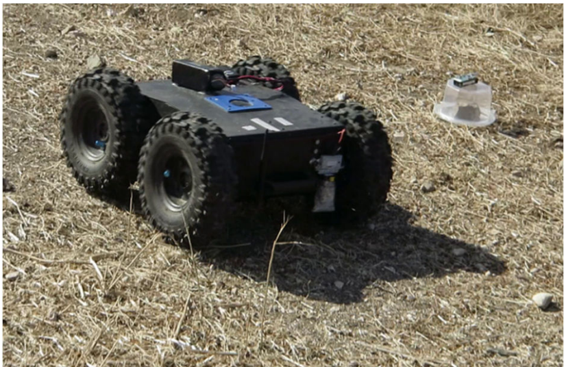
Figure 3: UGV approaches to a faulty sensor.
