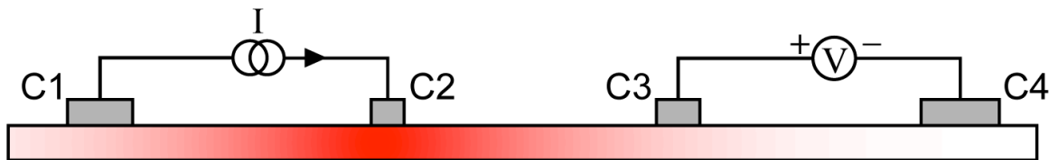
figure 1: In the 4-terminal non-local geometry we send a spin-polarized charge current from C2 (injector) to C1, we create a spin accumulation underneath C2. This drives a pure spin current in all directions, which can be detected by measuring the non-local resistance between C3 (detector) and C4.
