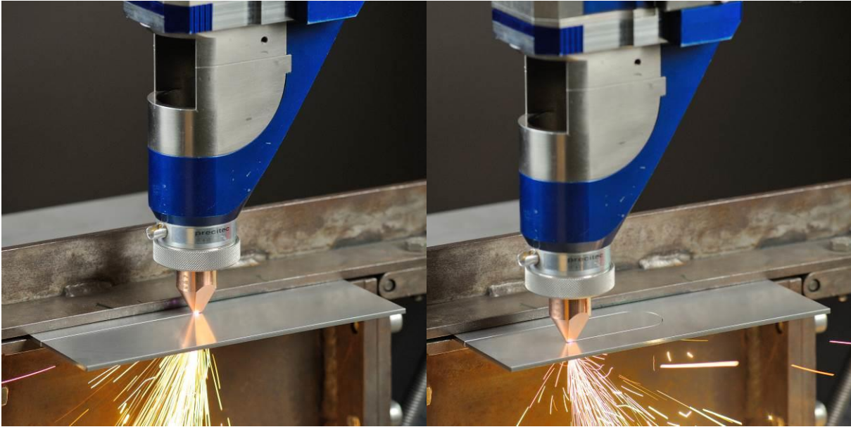
Fig. 34: Metal sheet cutting experiment (stainless steel, d = 2.5 mm, v = 18 mm/s, N_2 gas).
