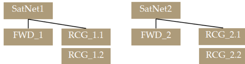
Figure 6.2 - Configuration logic of a SatNet and the configuration relationship between SATNET, forward links FWD_1 and FWD_2 and return link carrier groups (RCG).
