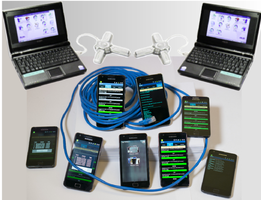
Figure 8: At the bottom, off-the-shelf Android devices running our protocol. At the top, two passive monitors with three antennas capturing environmental wireless traffic.
