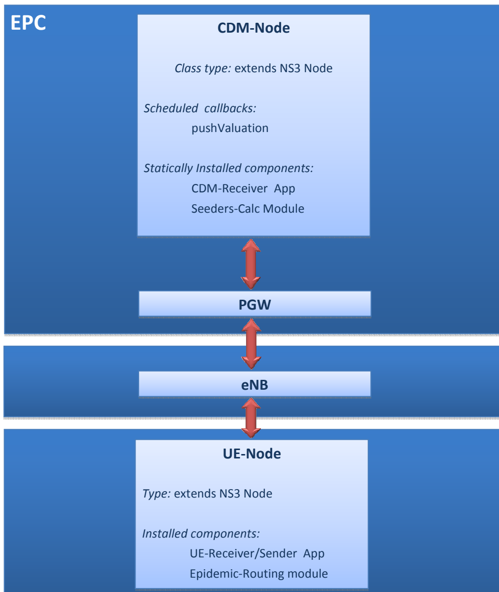
Figure 1: Push&Track software architecture model
