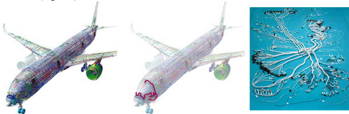
Figure 9: Main Routing Architecture Optimisation Research Experiment is aimed at reducing weight and cost for wiring systems for complex products such as aircraft
