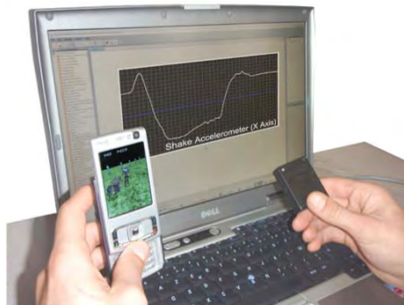
Figure 14: OIDE Debugging and Logging tools. In the example, the Shake accelerometer events are logged in order to tune the interaction with the mobile game.
