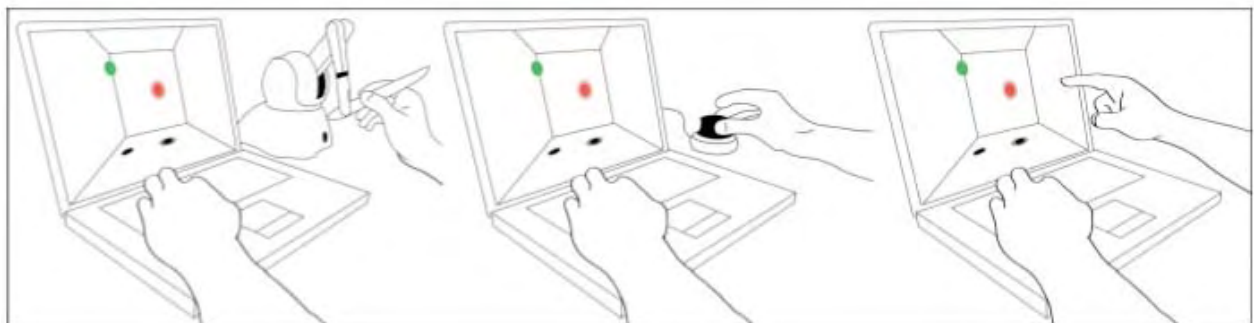
Figure 8: Experimental setting: Three configurations for the 3D pointing evaluation. Left: the PHANTOM, an arm-based device. Middle: the SpaceNavigator, a space-mouse. Right: AirMice technique, only fingers above the keyboard.
