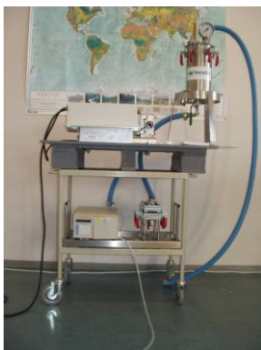
Figure 12 and 13. Images showing the pilot scale mobile membrane emulsification unit. The membrane is shown on the right figure.
