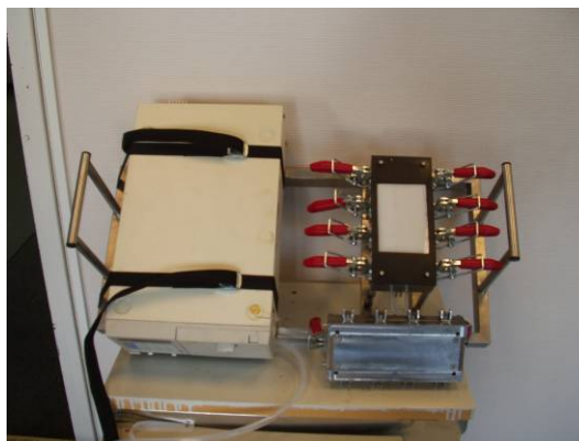
Figure 12 and 13. Images showing the pilot scale mobile membrane emulsification unit. The membrane is shown on the right figure.
