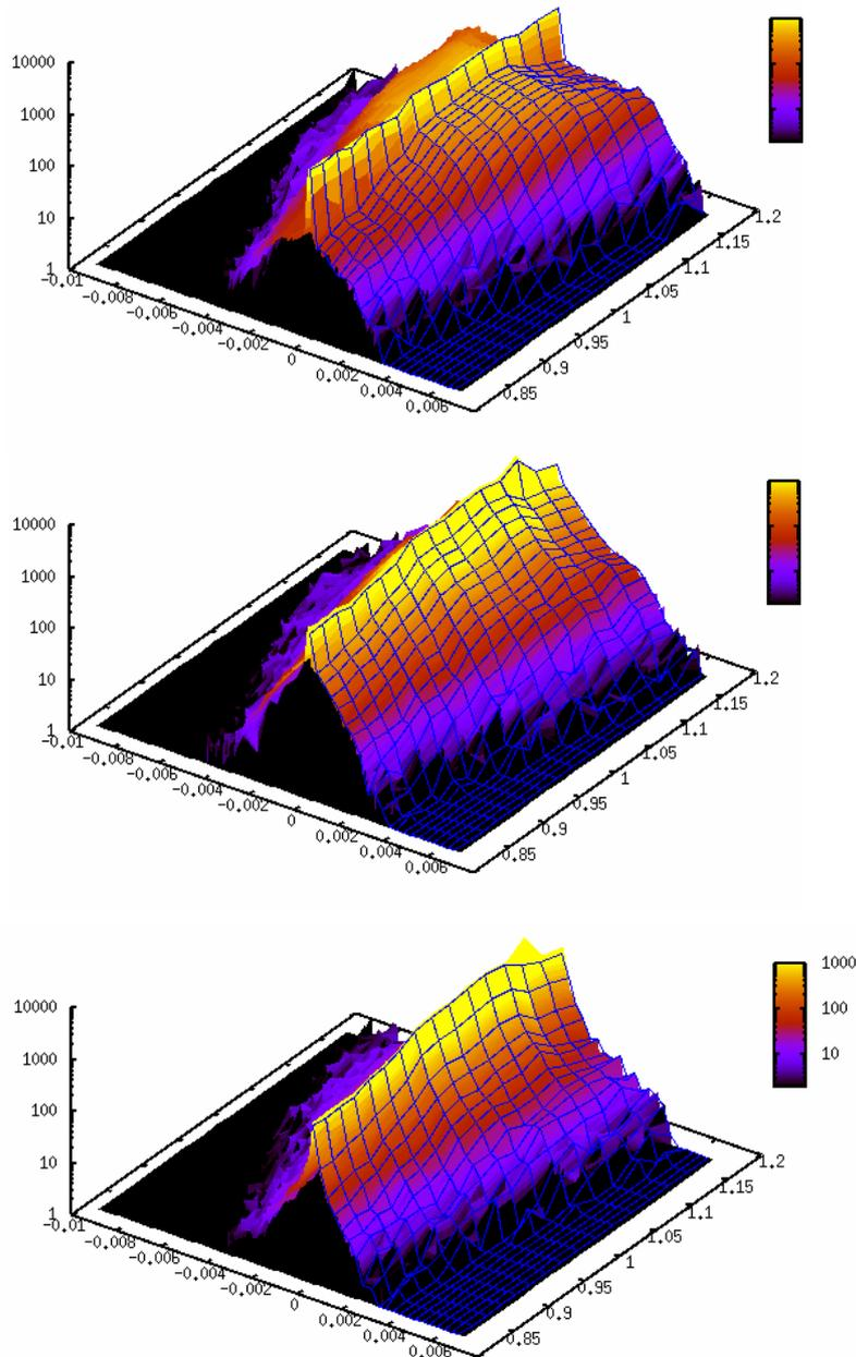
**Figure 12.** Off-specular 2D ( $\omega-2\theta$ ) SMR map, measured with the newly developed multi-APD array (time resolution 1 ns, pixel size 100 nm). The sample was an antiferromagnetically coupled Fe/Cr multilayer in the native domain state (top), after domain ripening (center) and after domain coarsening (bottom).
