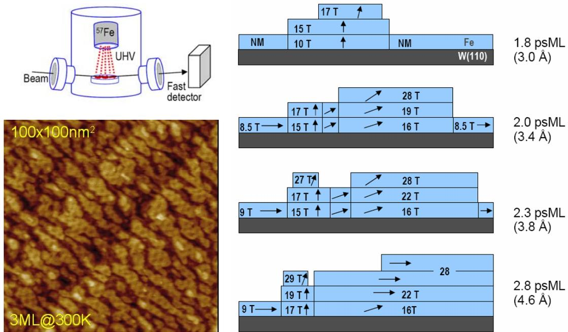
**Figure 10.** (top left) Geometry of the grazing incidence nuclear scattering (GI-NRS) UHV experiment at ID 18. (bottom left) STM image illustrating the growth mode for a 3 ML Fe film on W(110) (right) The spin structure derived from GI-NRS data shown for selected  $^{57}\text{Fe}$  coverage (in equivalents of pseudomorphic monolayers (psML)). The numbers indicate the layer values of the hyperfine magnetic fields. The layer resolved spin orientation is depicted by arrows.
