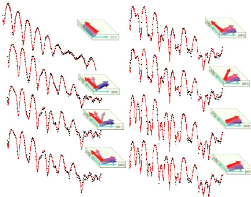
**Figure 11.** In-plane spin reorientation transition as seen by nuclear resonance scattering. The time spectra in the transition (from 23 ML, top left, to 25 ML, bottom right) are fitted using fan-like magnetization structures. as shown in the insets.
