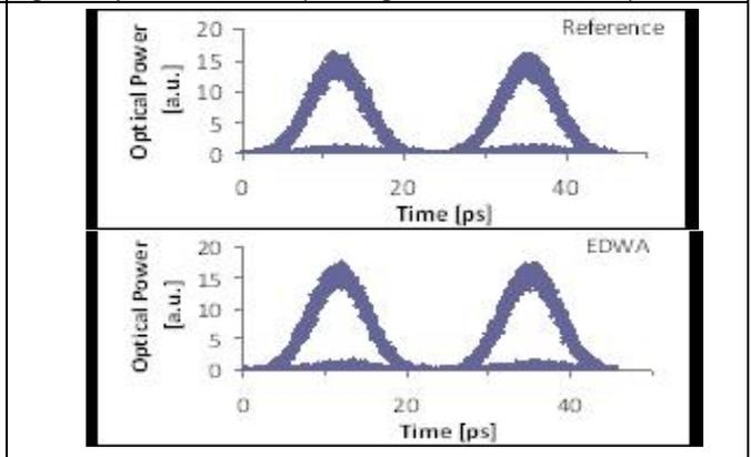
Fig. 9: Al<sub>2</sub>O<sub>3</sub>:Er<sup>3+</sup> amplifier response at 40 GBit/s data rate
