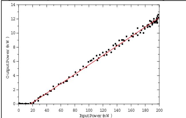
Fig. 8: Laser performance of 3%Yb<sup>3+</sup>:(Gd,Lu)<sub>2</sub>O<sub>3</sub> channel
