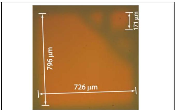
Fig. 7: Optical microscope image of local Al<sub>2</sub>O<sub>3</sub> deposition
