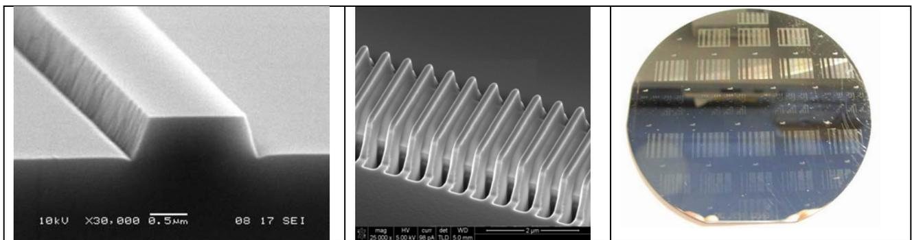
Fig. 3: 1.2- $\mu$ m-wide and 550-nm-deep channel in  $Al_2O_3$ Fig. 4: 23- $\mu$ m-long grating in  $Al_2O_3$  with 550-nm periodFig. 5: Wafer view of patterned HV-CVD-grown  $Al_2O_3$  waveguide
