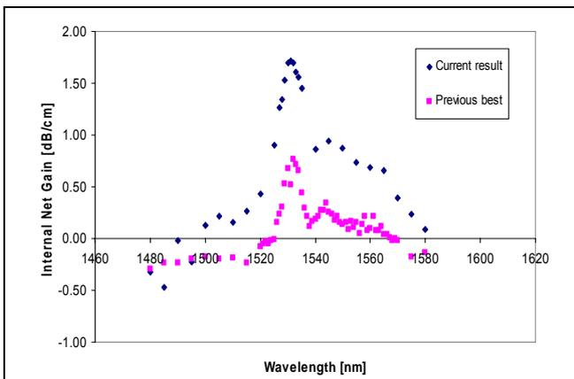
Fig. 6: Gain improvement in Er:Al<sub>2</sub>O<sub>3</sub> channel waveguides
