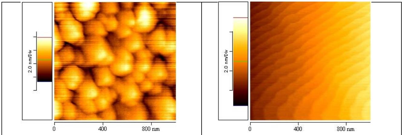
Fig. 1: AFM of 1- $\mu$ m-thick  $Sc_2O_3$  on  $Y_2O_3$  substrateFig. 2: AFM of 3.1- $\mu$ m-thick  $(Gd,Lu)_2O_3$  on  $Y_2O_3$
