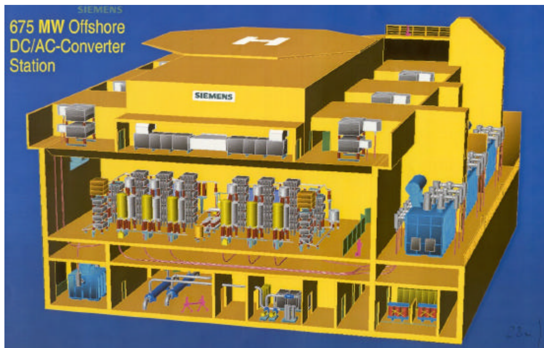
Figure 2.19 675 MW Siemens Offshore DC/AC-Converter Station
