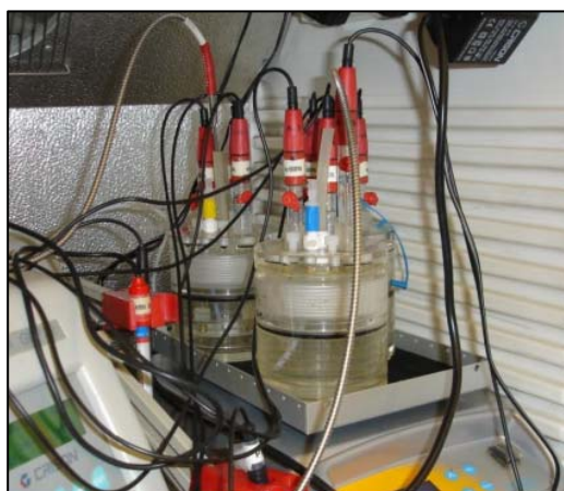
Experiments of consumption of dissolved oxygen by mineral as a function of time (Domènech et al., 2011, 3 rd ReCosy Annual Workshop)
