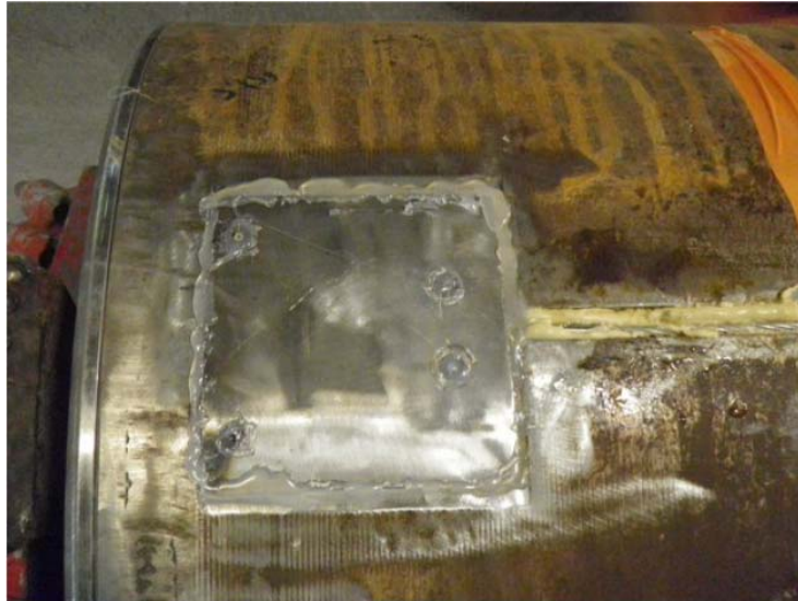
Figure 25: Capped inset holding the welded link between 2 optical fibres for measuring falls of blocks (front of casing element n°1)
