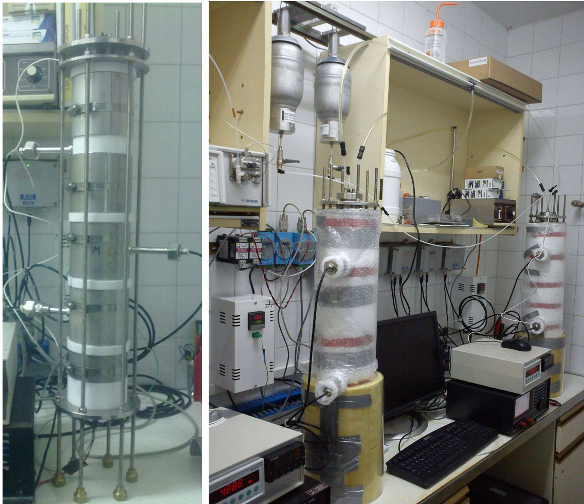
Figure 6: Cell B before being wrapped with the insulation material (left) and THM cells in operation (right)
