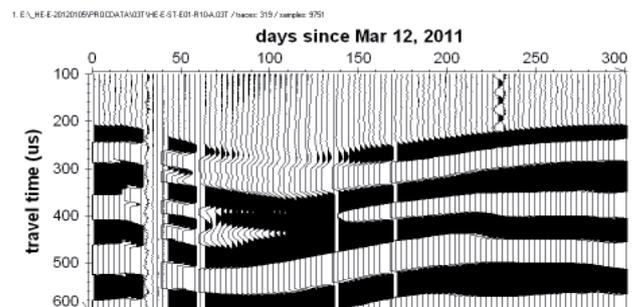
Figure 2. Seismic section recorded in the OPA at 10 cm distance from the interface OPA/SB. Only every third trace is plotted.
