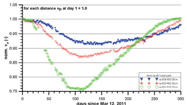
Figure 3. Normalised seismic P-wave velocities in the OPA at distances of 10 cm (green), 20 cm (red) and 30 cm (blue) from the interface OPA/SB.
