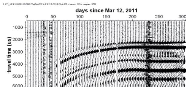
Figure 4. Seismic section recorded in the SB material between 5 cm and 10 cm from the interface SB/OPA. Only every third trace is plotted.
