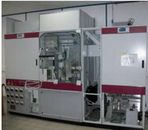
Figure 4.5 Automated cell culture system for massive amplification of pluripotent stem cells and their derivatives.
