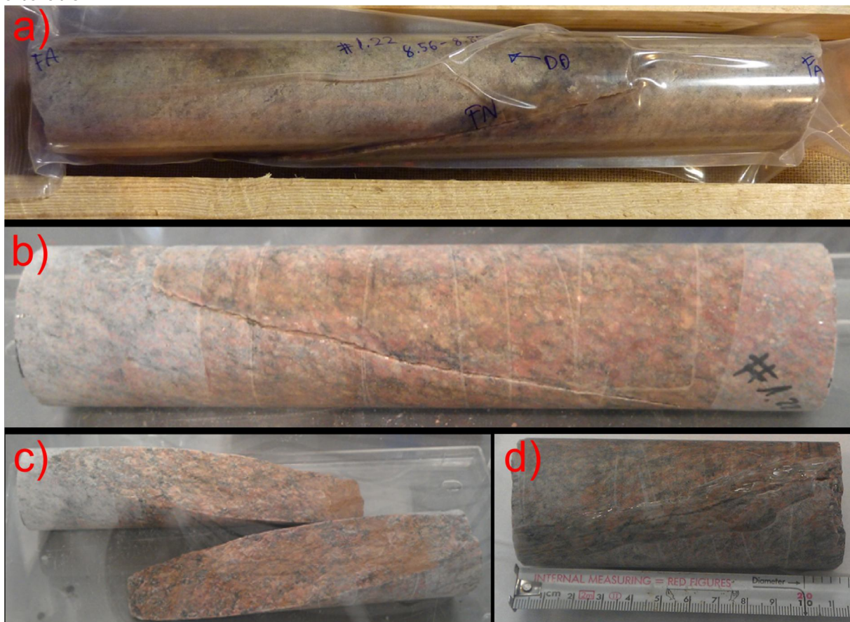
Figure 1: Core#1.22. a) Core as obtained during the drilling campaign under inert gas atmosphere. b) View of the fracture suture. c) Details on both fracture surfaces showing a coating of reddish mineral phases. d) Core as prepared before gluing into the Plexiglas cylinder.
