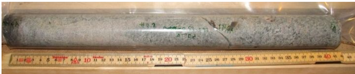
Figure 3: Drill core section #2.2 (0.53-0.97 m) from drill hole KA2370A-01 with a natural fracture.
