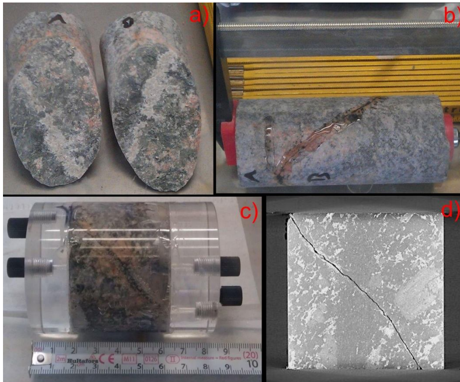
Figure 4: Core#2.2. a) Details on both fracture surfaces. b) Core as prepared before gluing into the Plexiglas cylinder. c) Core after preparation fitted with tubing ready for CT measurements and the migration experiments. d) CT slice of the core showing the open fracture (black line from bottom right to upper left).
