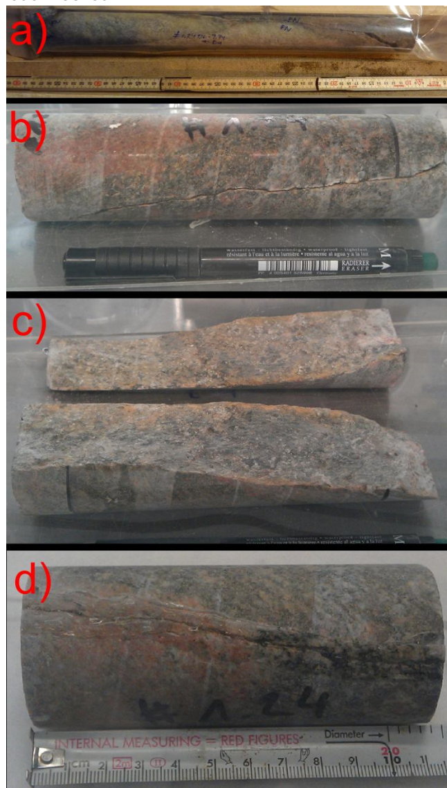
Figure 2: Core#1.24. a) Core as obtained during the drilling campaign under inert gas atmosphere. b) View of the fracture suture. c) Details on both fracture surfaces. d) Core as prepared before gluing into the Plexiglas cylinder.
