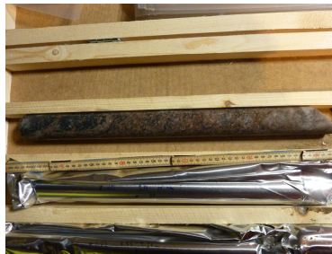
Crystalline rock drill core sealed in LD-PE bag and second confinement by Al bag, sampled at Äspö for the CP CROCK (Schäfer et al., 2012).
