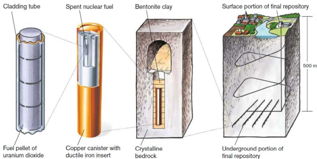
**Figure 1:** The KBS-3 concept for disposal of spent nuclear fuel (SKB 2011)
