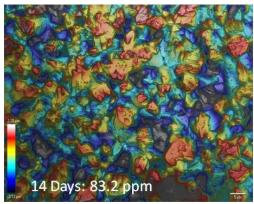
Figure 1. Optical Profilometry of polished CeO<sub>2</sub> monolith after 14 days at 150 °C in 2M HCl.
