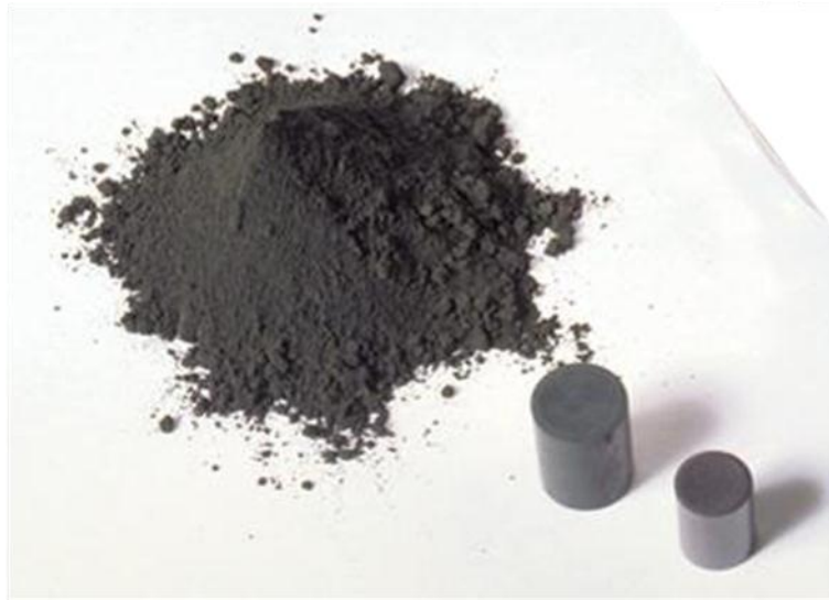
Fig. 1 From powder to pellet: Grain Size: \text{UO}_2 : \varnothing 20\text{ }\mu\text{m} , Pellet dimensions: PWR 17\times 17 : \varnothing 8.17 (AREVA), L 9.8 mm, BWR 10\times 10 : \varnothing 8.87 (Atrium 10XP), L: 10.5 mm
