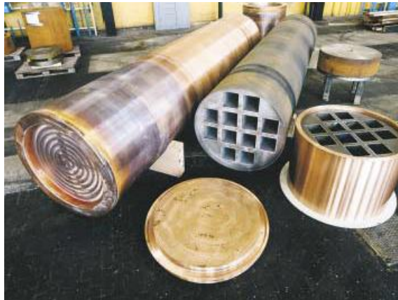
Fig. 9 Components of the Swedish canister concept at SKB's Canister Laboratory in Oskarshamn.
