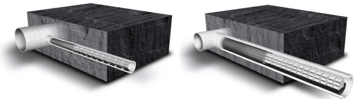
Fig. 6. Artist impression of the disposal cells for HLW (left) and LILW (right)
