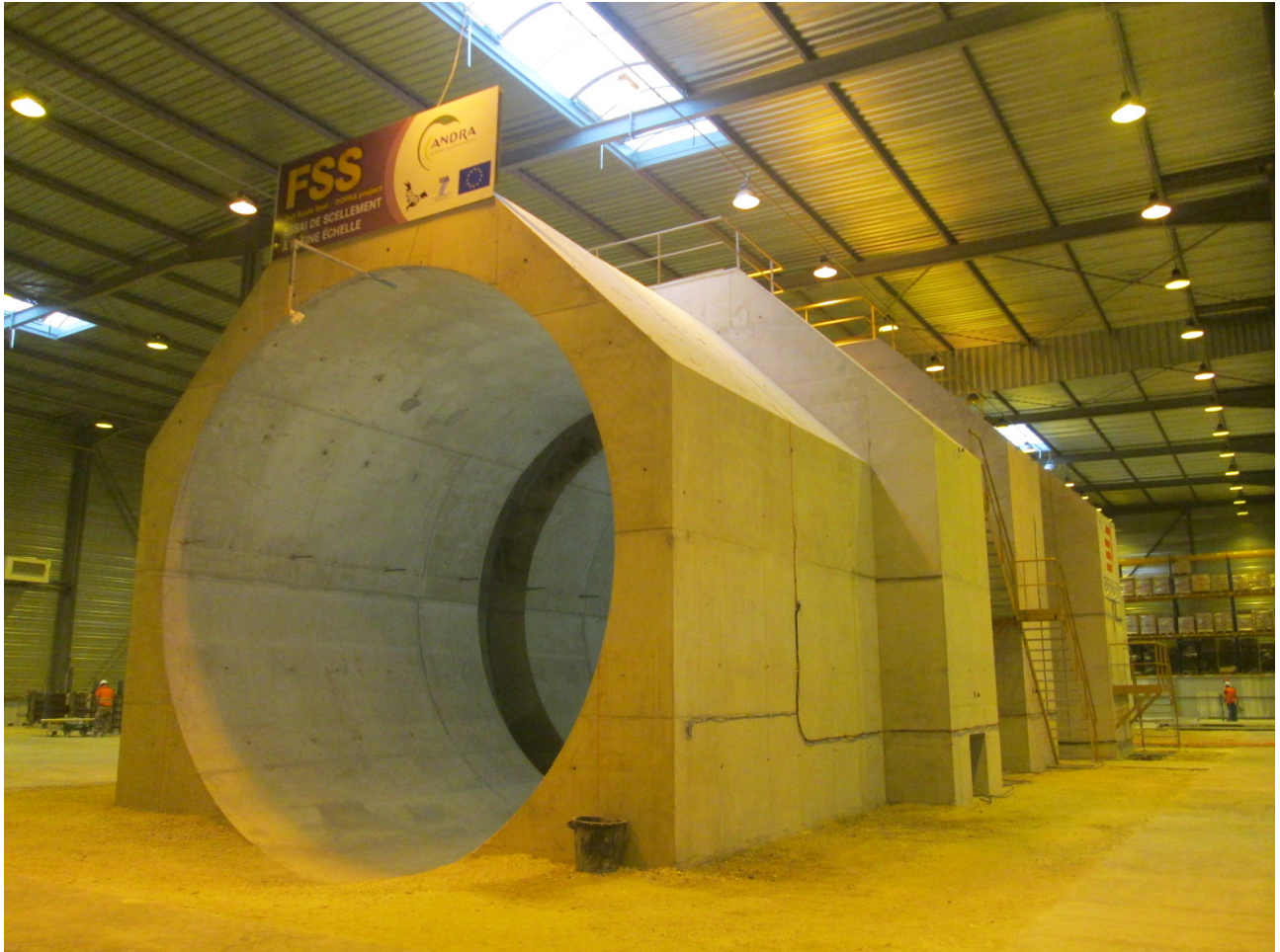
Picture 1. Full-scale text box constructed are ready for FSS Experiment (Photo: Andra)
