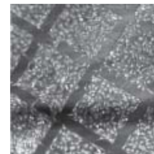
Figure 1. Optical microscope picture of the fibroblasts growing selectively in the fouling areas on a fouling-antifouling surface micropatterned by optical lithography.
