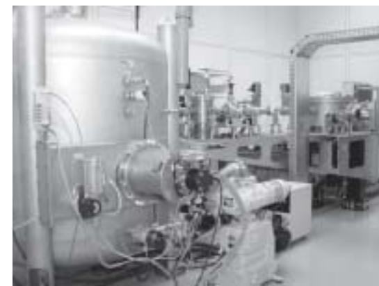
Fig. 2: Photograph of the laboratory EUV reflectometer. From the left to the right the following modules are shown: 1: goniometer chamber for large samples, 2: beamline with beam splitter, filters and monochromator and 3: chamber with the EUV source.
