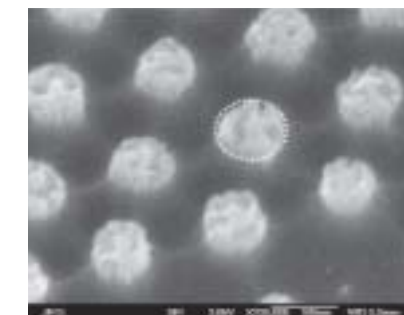
Figure 2. Scanning Electron Microscope picture of the proteins selectively absorbed on the polymeric nano-structures. The center of each dome is COOH-functionalized surrounded by anti-fouling matrix with a hexagonal arrangement: the bright objects in the picture (one indicated with a red circle) are the proteins.
