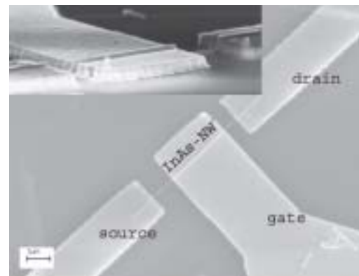
Fig. 1. SEM image of an omega-shaped gate n-InAs nanowire-FET.
