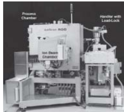
Fig. 2: General view of the IonScan 800
