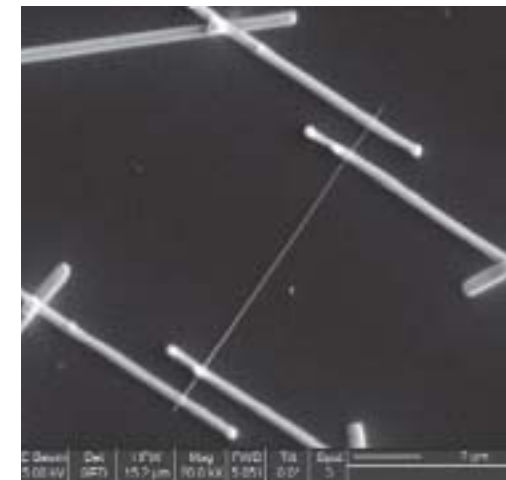
Fig. 1 SEM image of a nanowire-based FET over a micromachined substrate
