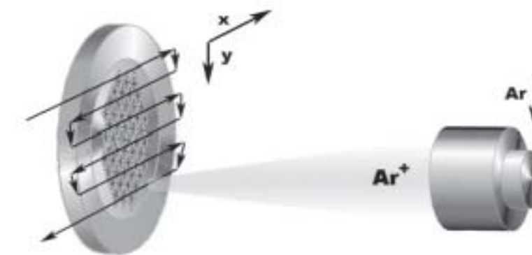
Fig. 1: Function diagram of film thickness trimming controlled upon residence time
